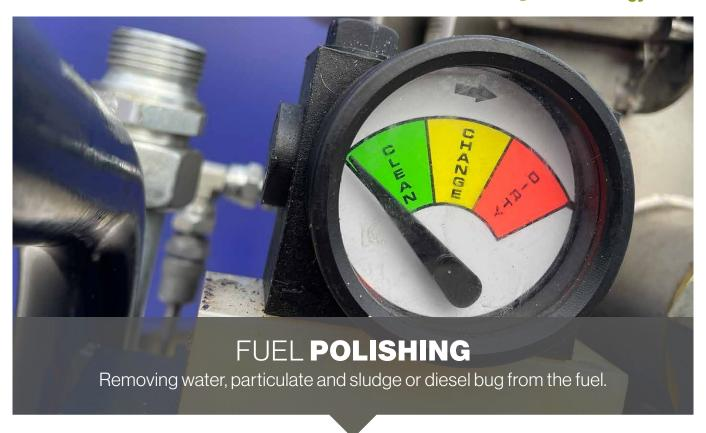
Fuel polishing is an advanced mechanical fuel cleaning process. Our service removes water, sludge particulates and microbial contamination from fuel in tanks and our knowledge and expertise guarantee limited disruption and downtime to your business.
